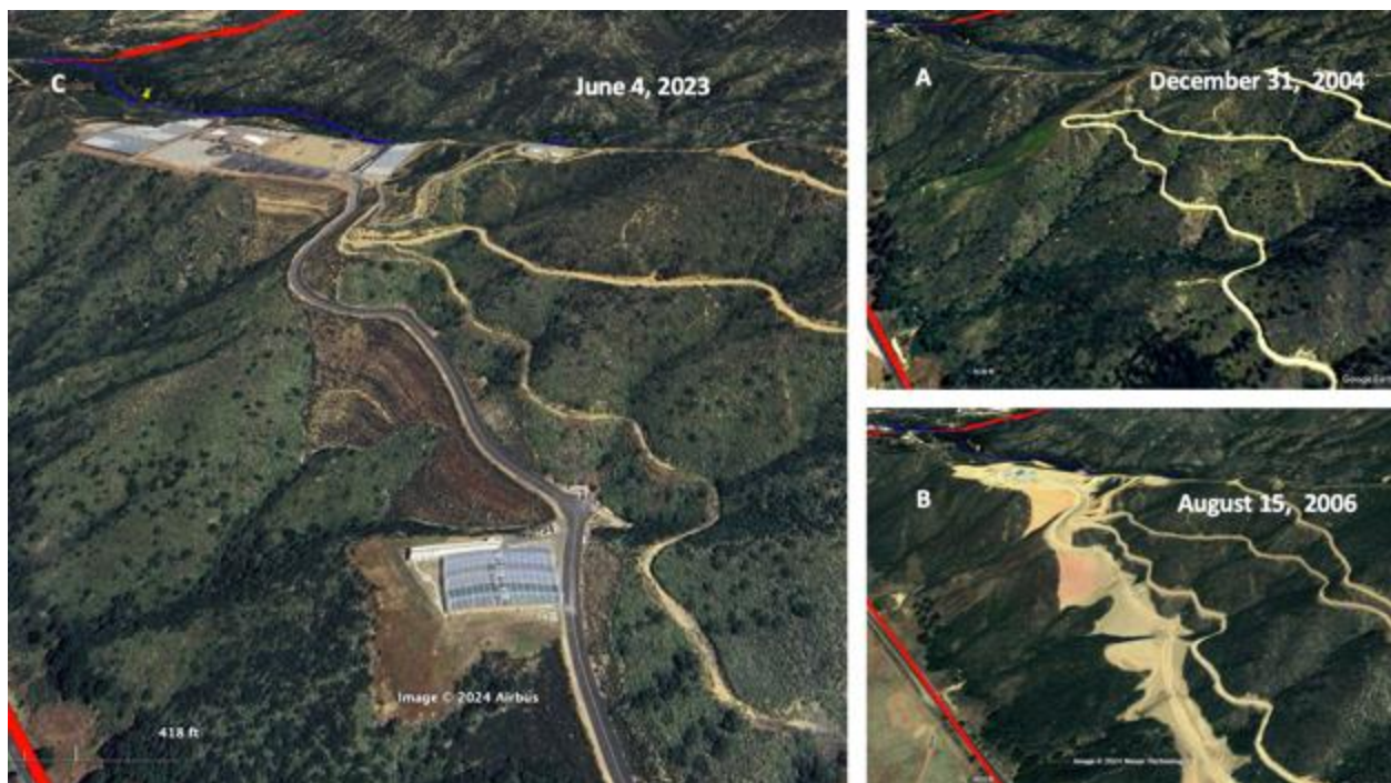
Figure 6. Sediment and water are/are not in balance. Excess sediment is generated at the start of construction in 2004 as part of road development on the hill. In 2006, slope stabilization and cutting of construction pad. In 2023, plants stabilize the hillslope, but the creation of roads and development structures increase water flow from impervious surfaces. A. December 31, 2004, Maxa Technologies; B. August 15, 2006, Maxar Technologies; C. June 23, 2023, Airbus. All images are from Google Earth.
